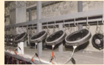
Speaker Accelerated Life Test
